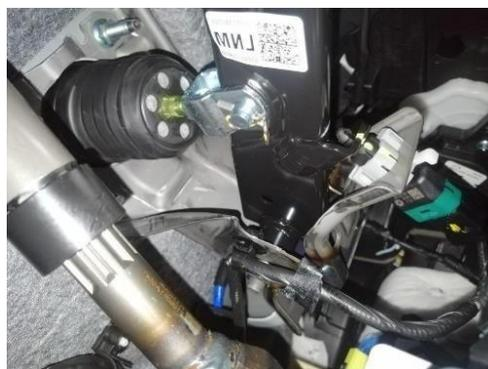
**Figura 53: sensor de pedal**
